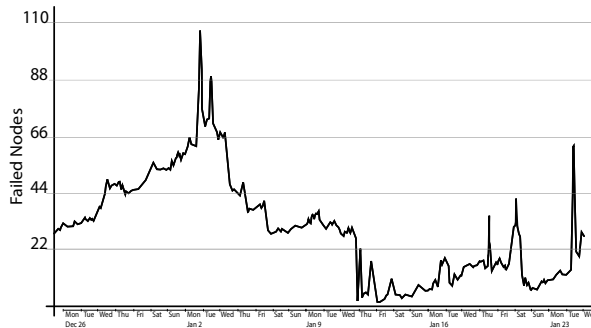
Figure 1: Number of failed nodes over a single month period in a 3000 node production cluster of Facebook.
